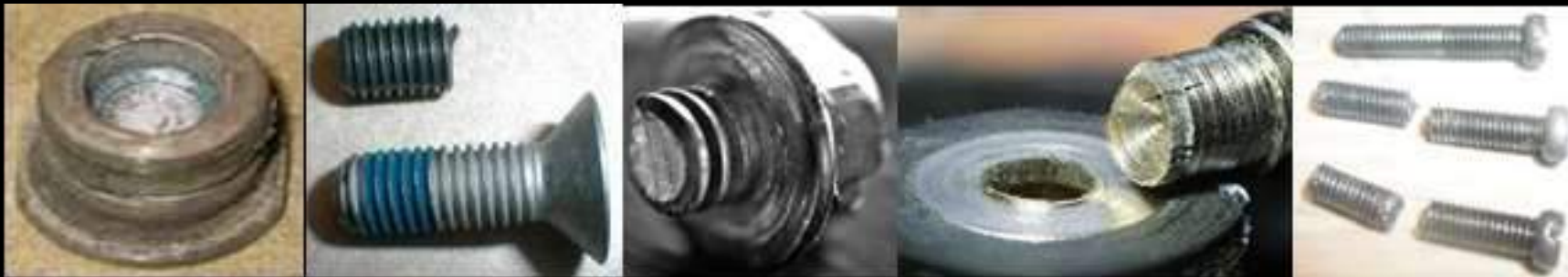
Broken and spoiled screw
