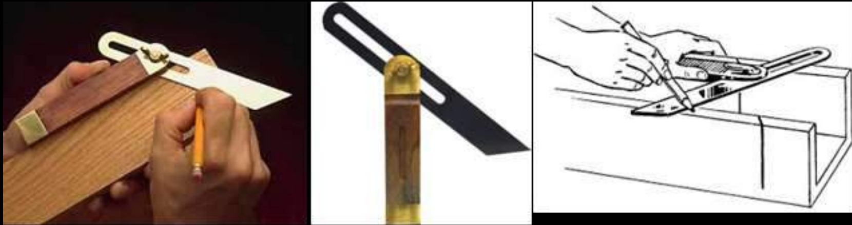
Bevel gauge and its use
