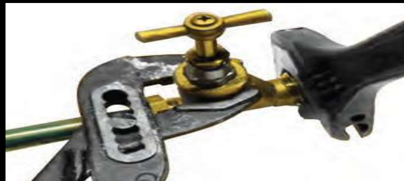
Opening of a compression nut
