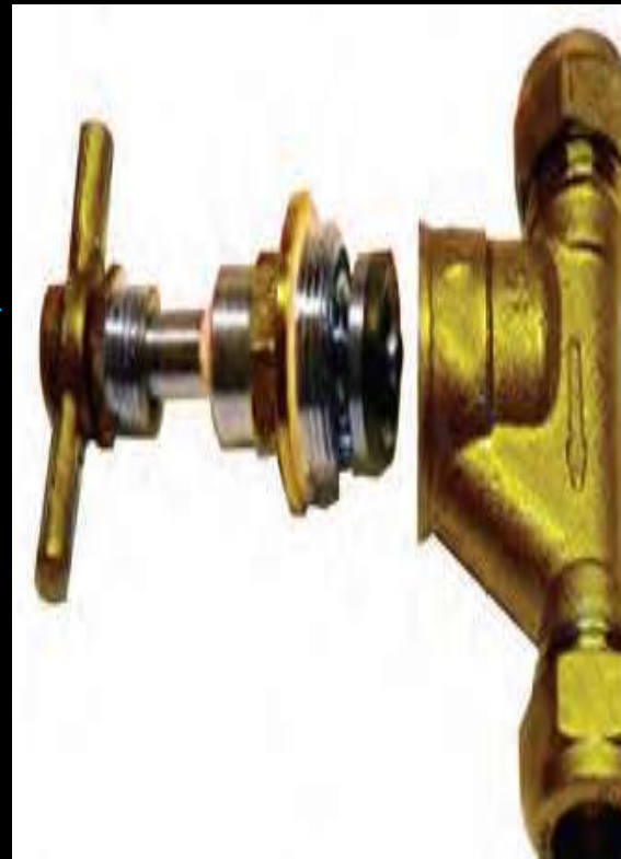
(b) Separating body of a tap
