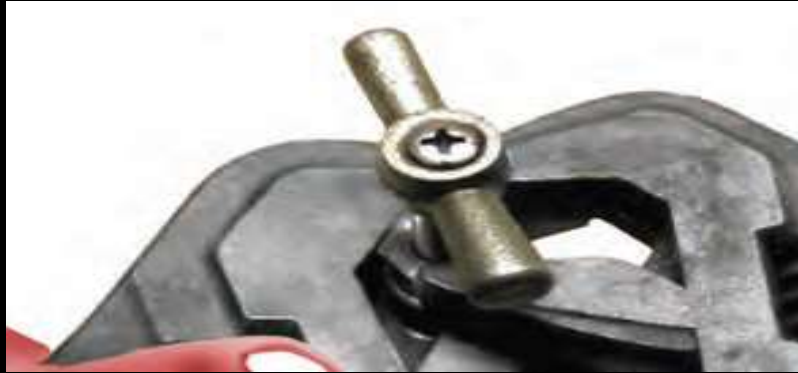
Tightening of a gland nut
