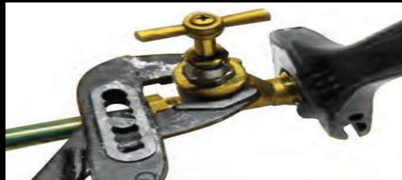
Opening of a compression nut
