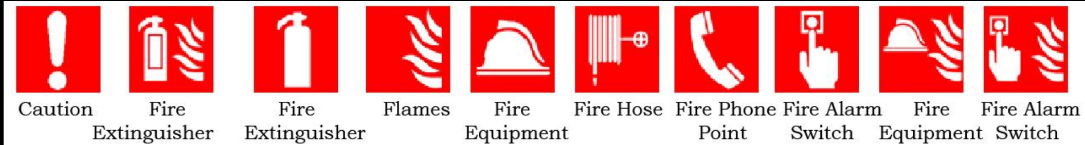
Fig. Fire Equipment Symbol
