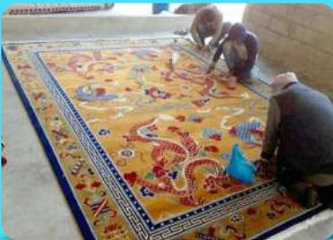
Singeing is the process of burning protruding fibers. And this done on the back side of the carpet to give it a sharp and neat finish.
