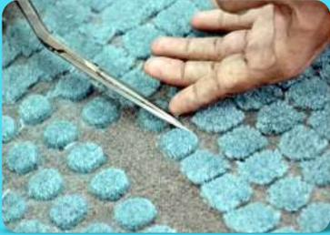
Once the carpet is cleaned and dried, the piles of the fabric are cut to level the overall height by the process of shearing. This followed by the process of embossing, in which the piles of the border of the motif are cut lower than the body of the motif. It is followed to give a good look to the carpet, as the motif seems to be protruding out of the background.
