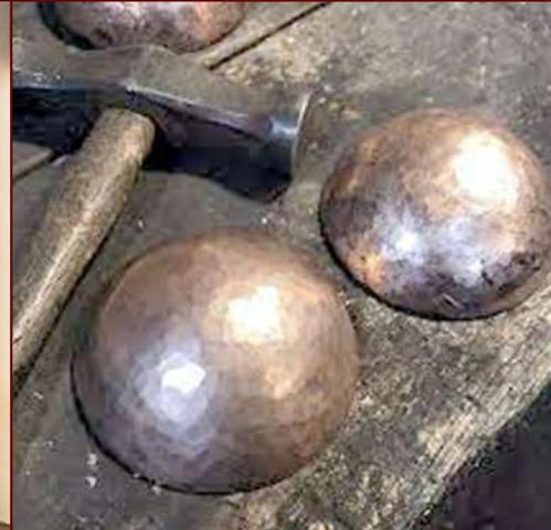
The individual at work is responsible to hammer holes and designs on the surface of the metal as per the design and requirement. The individual at work is responsible to remove excess metal from the product. The person reshapes, resizes and smoothens the metal product as per the design and requirement. The job requires the individual to have: attention to details, good eyesight, steady hands, ability to sit in same position for longer hours and patience.
