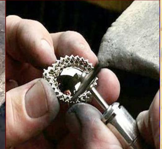
The individual at work is responsible to polish and provide finishing to the metal surface as per requirements with appropriate abrasives. The polisher is also responsible to clean the workplace subsequently. The job requires the individual to have: attention to details, good eyesight, steady hands, ability to sit in same position for longer hours and patience.
