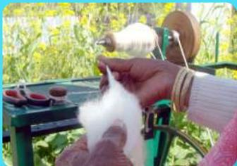
The fibers accumulated and cleaned in previous stages, are now arranged to form woollen yarns. This stage consists two steps- Carding and Spinning. Carding aligns the fibers in one direction. It is performed by hand by the help of a carding brush or rollers. Then finally the carded wool is spun into yarn using a spinning wheel or charkha
