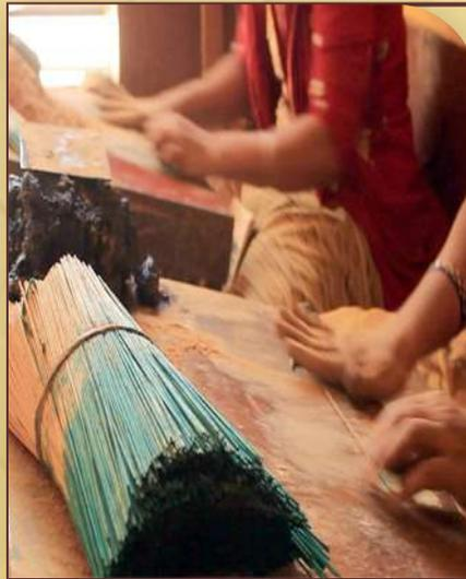
Agarbatti Maker is the one who produces agarbatti (perfumed or un-perfumed depending on ingredients) by rolling agarbatti masala dough over bamboo stick manually using hand. The major ingredient for hand rolled agarbatti are bamboo stick and agarbatti masala preparing bamboo stick for rolling preparing agarbatti masala dough
