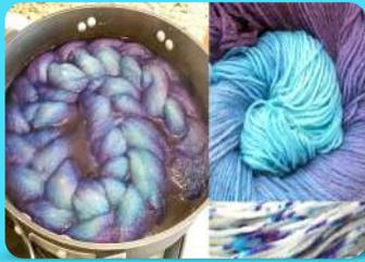
Dyeing helps in incorporating colours into the yarns. Mechanical dyeing is performed in closed chambers through standardized methods, using dyes from international manufacturers. Though the initial traditional pot dyeing method has been recently replaced, few artisans still follow this technique. Colourful yarns with high degree of fastness is achieved after it is dried for one to three days the yarns are sun-dried, depending on weather
