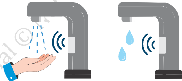
Fig. 1.19: Touch-Activated sensor faucets
