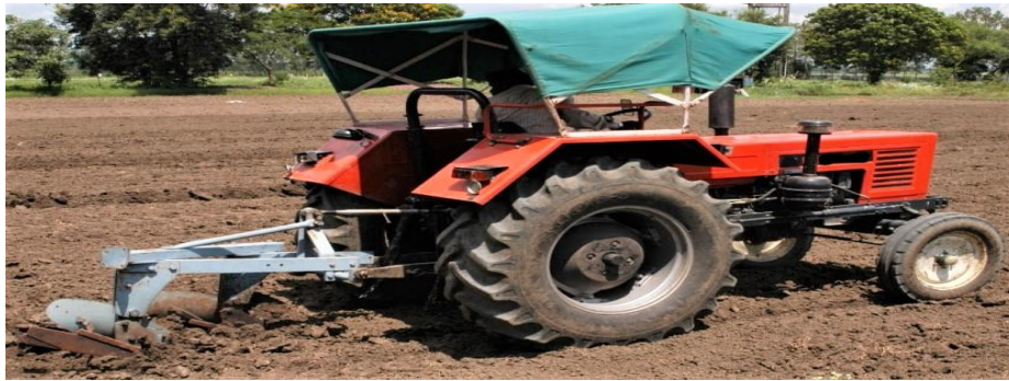
Fig. 3.10: Field operation of MB Plough
