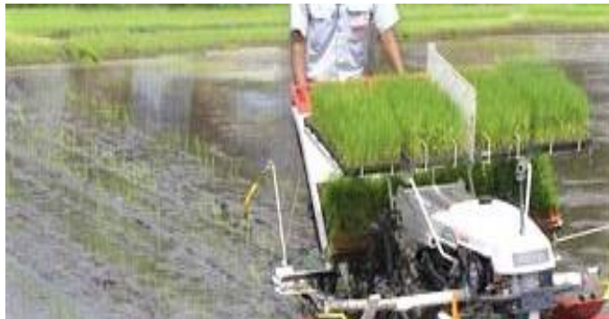
Fig.3.38: Self-Propelled walking type rice transplanter (2-wheel)
