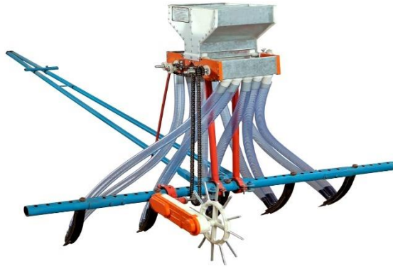
Fig.1.23: Bullock drawn seed-drill with metering unit
