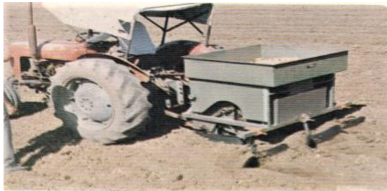
Fig.3.41: Potato planting using semi-automatic potato planter
