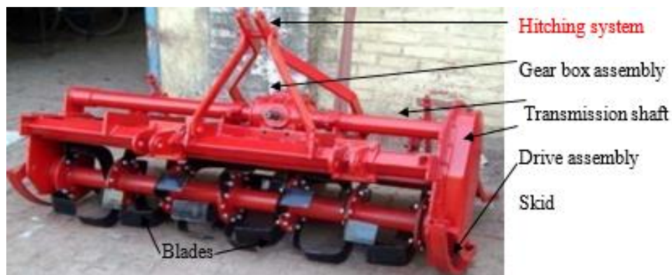
Fig.3.16: Rotavator and its major parts
