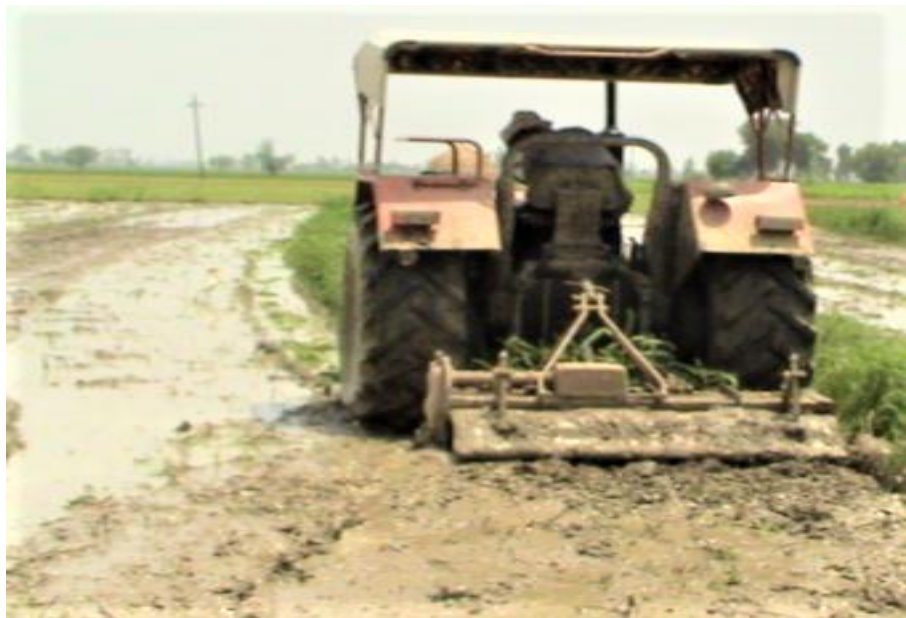
Fig. 3.18: Field Operation with Rotavator (Wet Condition)
