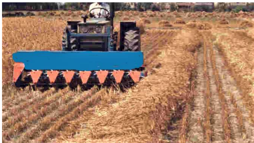
Fig.3.58: Tractor front mounted vertical conveyor reaper-cum- windrower
