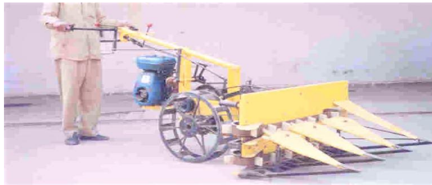
Fig.3.57: Self-propelled vertical conveyor reaper-cum-windrower
