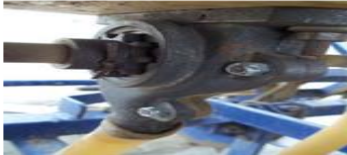
Fig. 3.30: Fluted Roller Seed Metering
