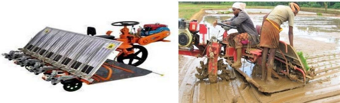
Fig.3.39: Riding Type - Self Propelled Rice Transplanter (three-wheel)
