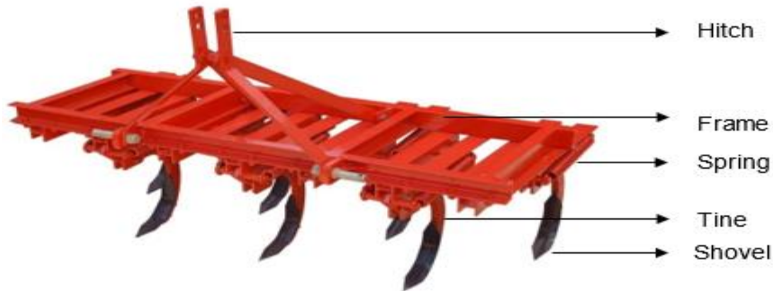
Fig.3.22: Spring Tine Cultivator
