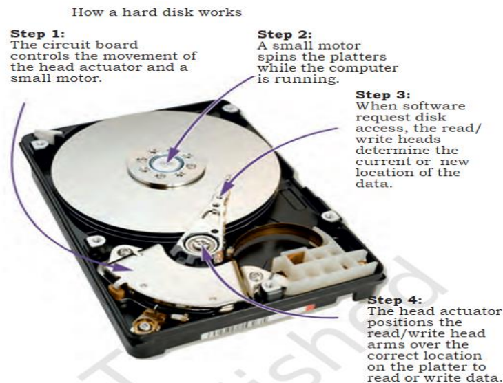
Fig. 3.11 working of hard disk
