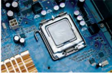
Fig.2.11: Installing CPU on the motherboard
