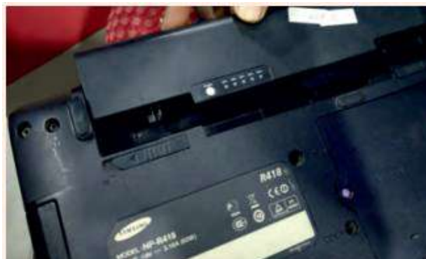
Fig. 4.16 Remove battery and optical drive
