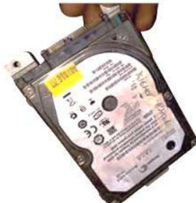
Fig. 4.19 Remove old hard drive assembly
