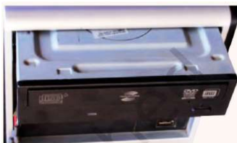
Fig. 4.22 Insert optical drive
