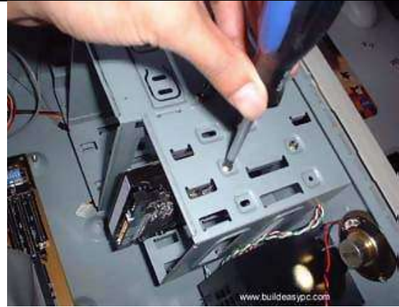
Fig. 4.10 Fit the Hard drive in case on Fig. 4.11 Screwing the hard disk drive proper place
