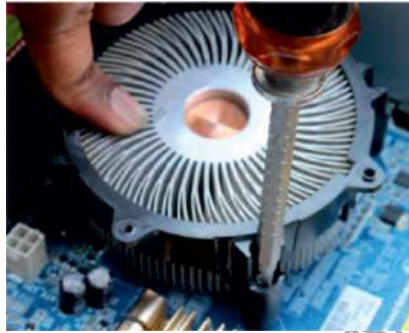
Fig. 2.14.: Screwing the heat sink
