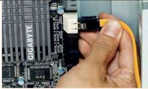
Fig. 4.15 Plugging SATA data cable into the motherboard
