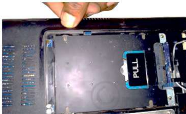
Fig. 4.18 Open connector and release hard drive cable
