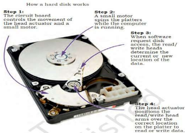
Fig. 4.9 working of hard disk
