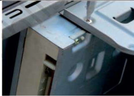
Fig. 4.23 Tighten screws of optical drive
