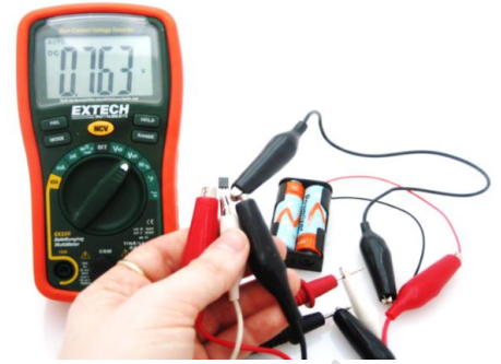
Fig.2: TMP36 sensor testing at room temperature
