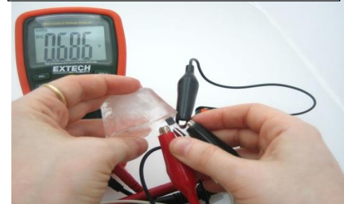
Fig.4: TMP36 sensor testing at low temperature
