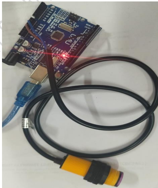
Fig .1: Proximity Sensor to Arduino UNO Circuit Connection
