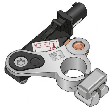
Fig.2.42: Current, voltage, and battery sensor
