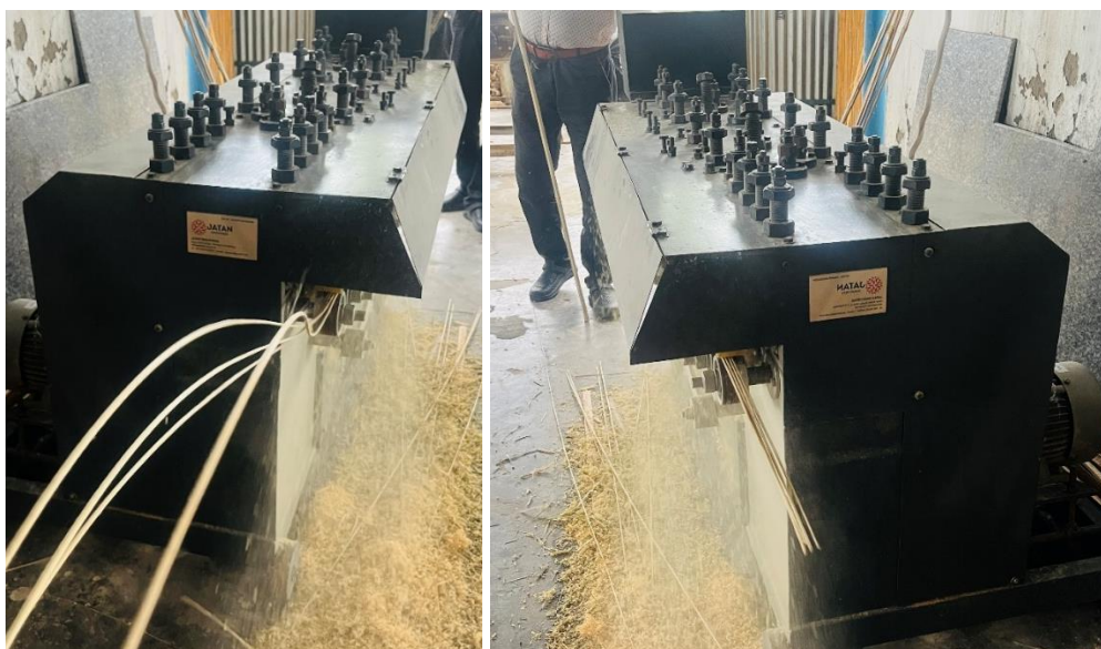
Fig. 3.2: Bamboo sliver making using slivering machine
