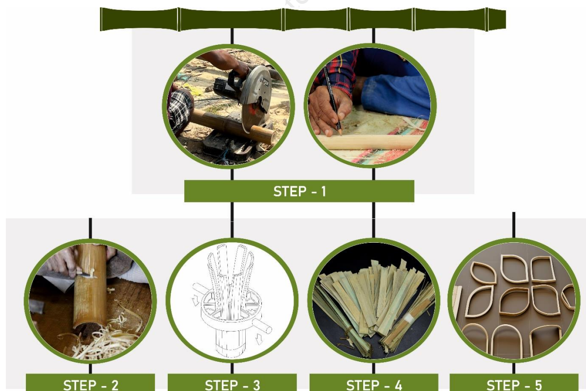
Fig. 3.34: Steps involved in bending of bamboo
