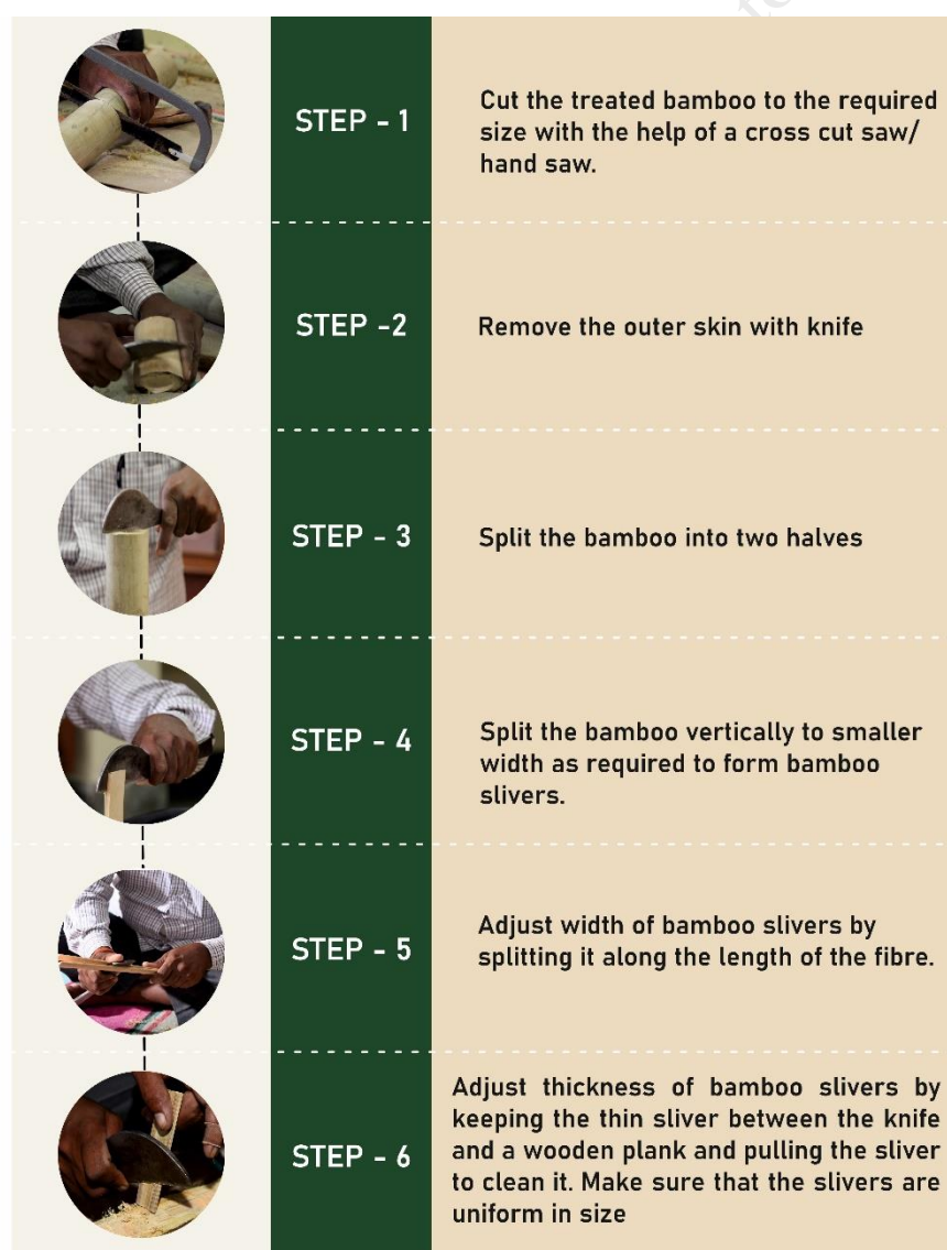
Fig. 3.1: Bamboo sliver making process using saw
