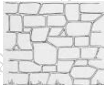
Fig.1.9: Uncoursed Rubble Masonry
