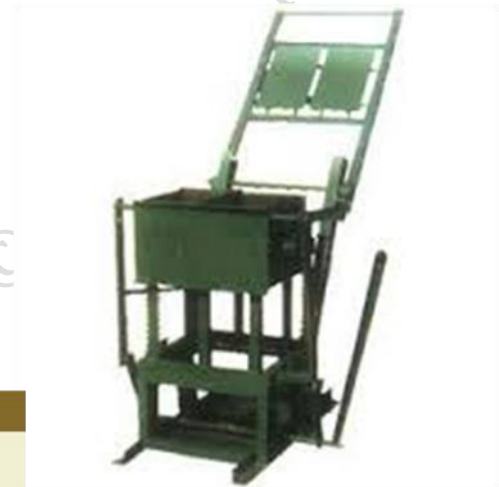
Fig.4.6: Block casting machine
