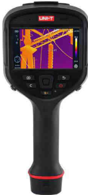
Figure-4.1: Handheld professional thermal imaging infrared (IR) camera displaying a thermal image on its screen
