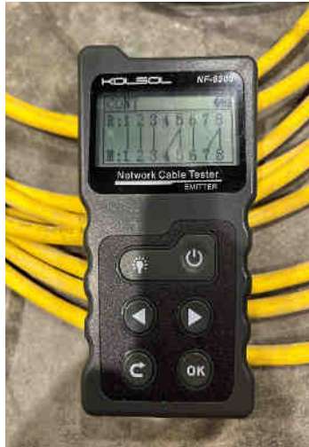
Figure- 5: Network cable tester LED display showing continuity test results for pins 1 to 8 on both receiver and emitter sides (Reference: https://www.reddit.com/r/HomeNetworking/comments/16n4dot/what_does_this_ethernet_continuity_test_result/ )
