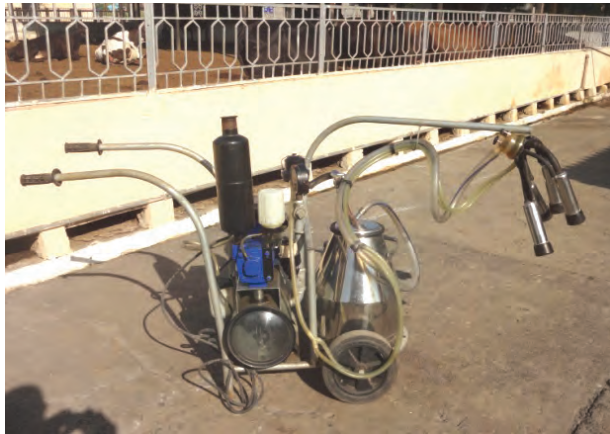
Fig. 3.14(a): A mobile automatic milking machine
