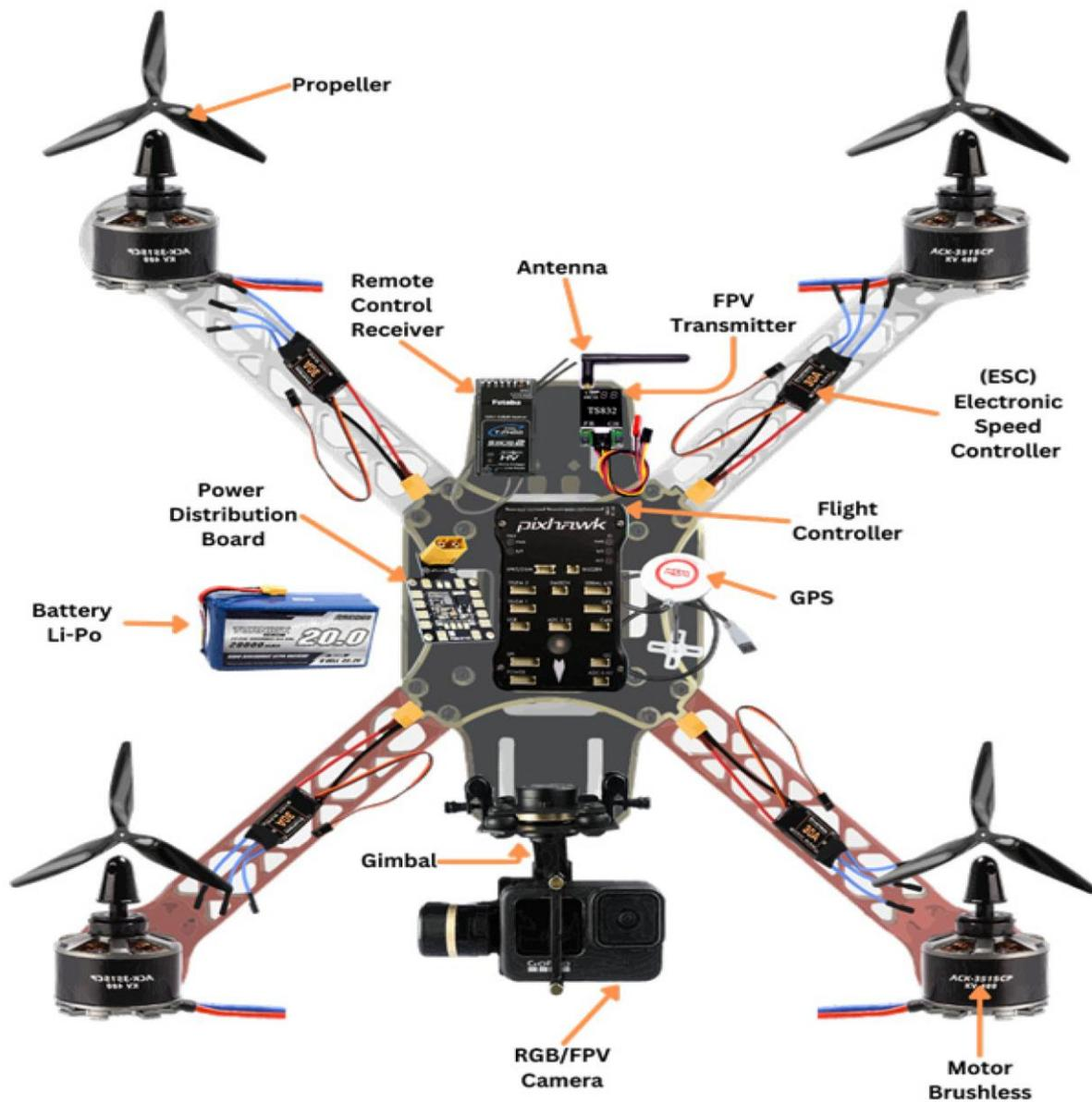
Fig. 1.1 Drone Parts
