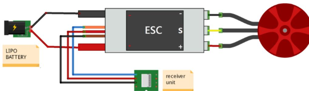
Fig. 1.6 Line diagram of Electronic Speed Controllers
