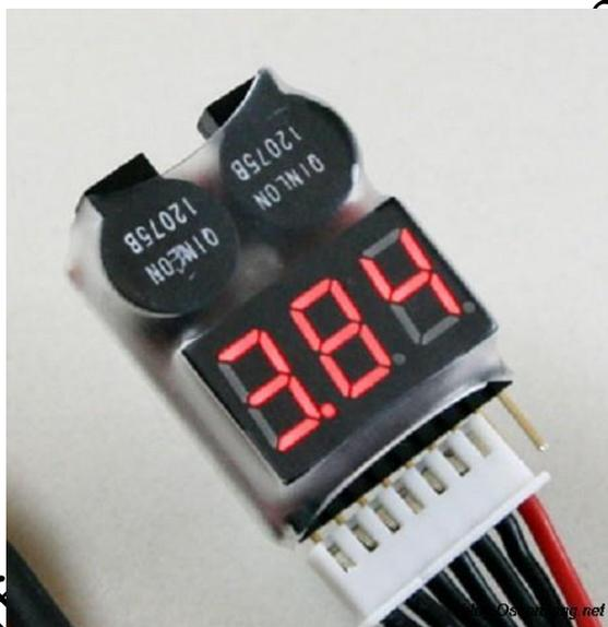
**Fig. 2.1 Battery check by battery Tester**
