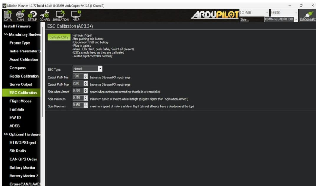
Fig. 1.21 ESC Calibration
