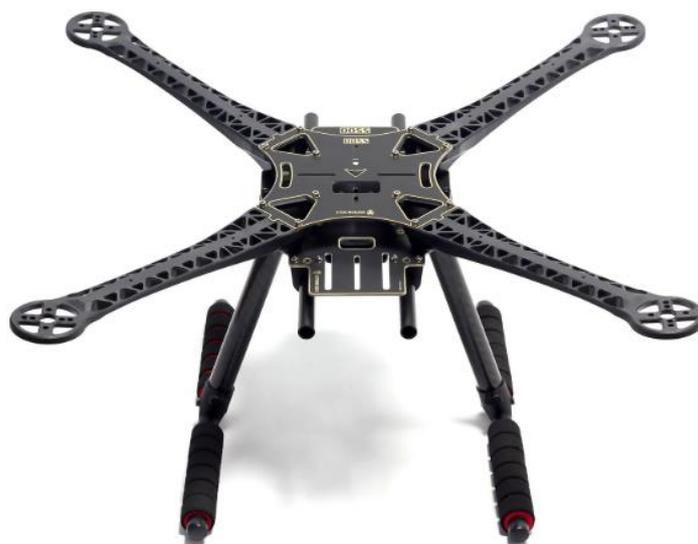
Fig. 1.3 Drone frame and landing gear
