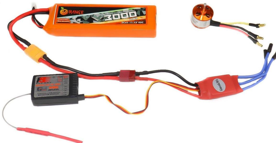
Fig. 1.7 Electronic Speed Controllers
