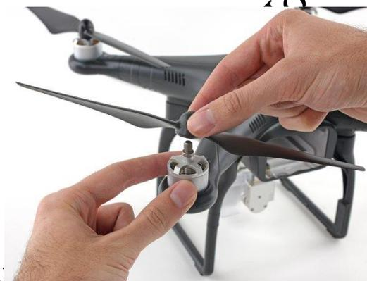
**Fig. 1.24 Remove the Propellers**
