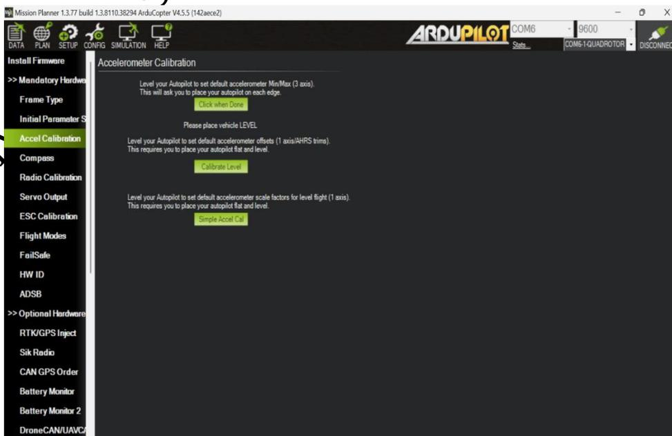
Fig. 1.17 Accelerometer Calibration
