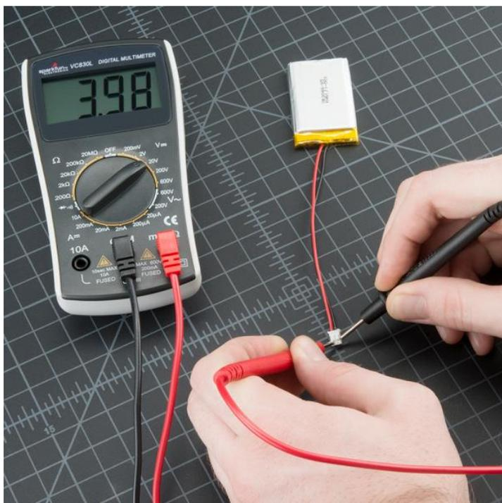
**Fig. 2.2 Battery check by Multimeter**
