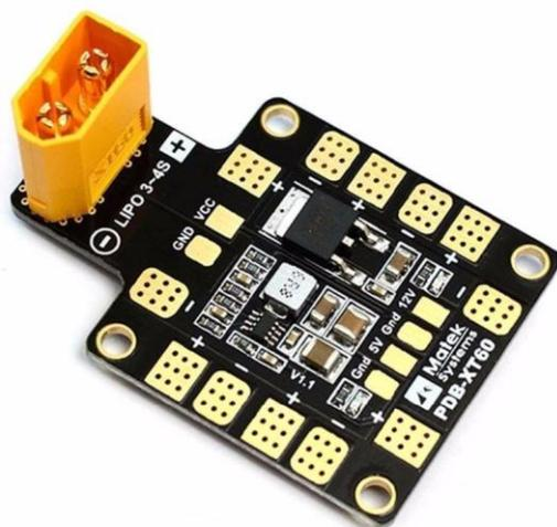
Fig. 1.9 Install Power Distribution Board
