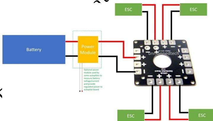
Fig. 1.10 wiring diagram of Power Distribution Board
