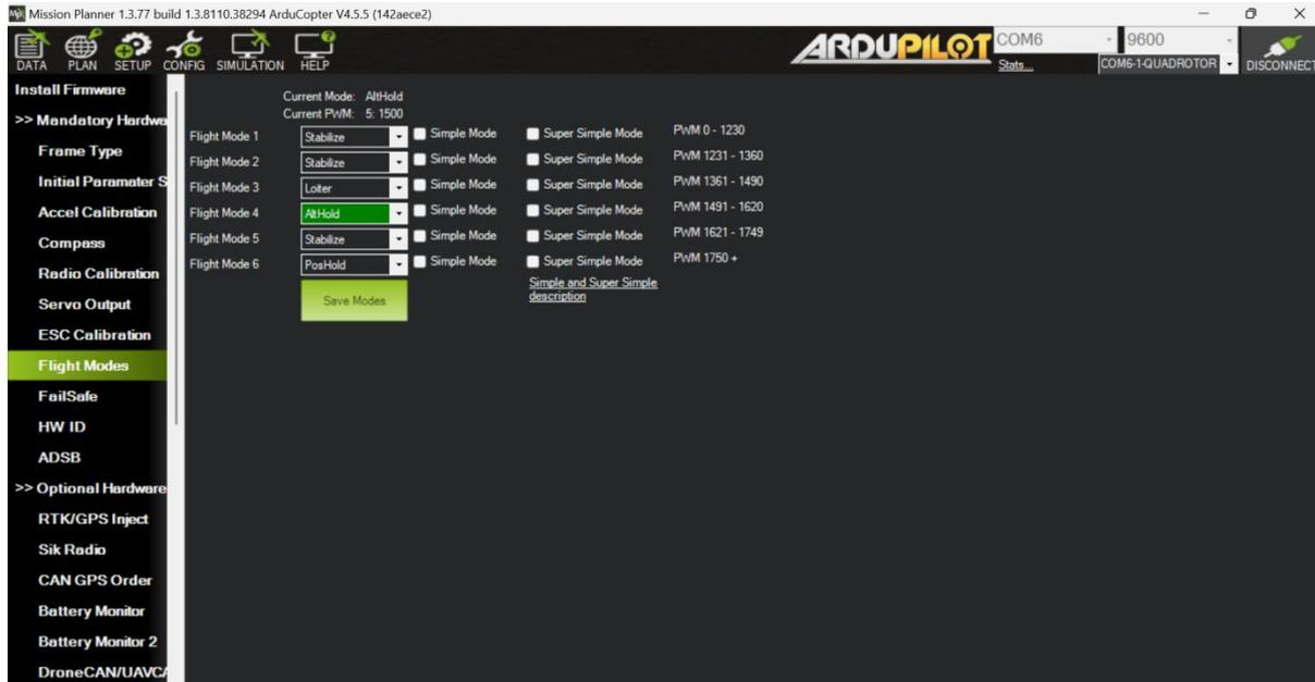
Fig. 1.22 Flight Mode Setup
