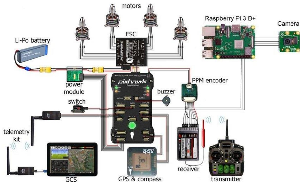
Fig. 1.12 wiring connection of drone
