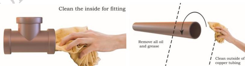
**Fig. 3.37 Cleaning of copper tube**
