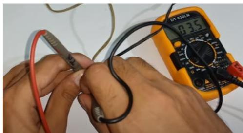
**Fig. 2.84 Resistance of the temperature sensor on the display**
