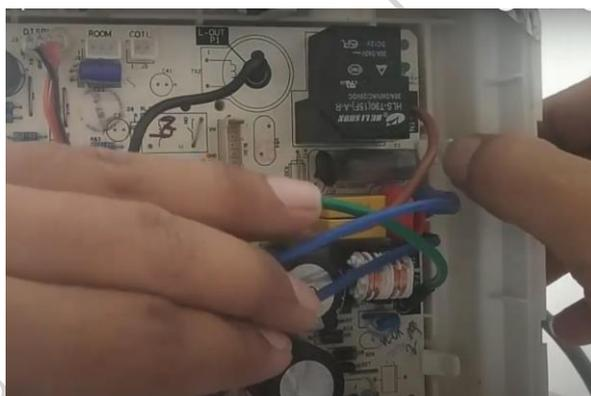
**Fig. 3.26 Side clip removal**
