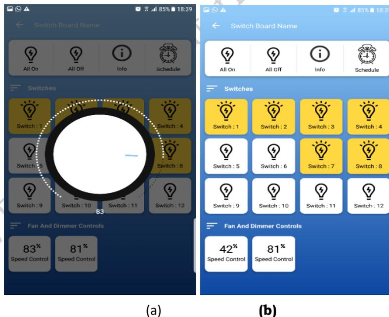
**Fig. 5.11 (a) Regulator to control the speed of fan, (b) Dimmer control**
