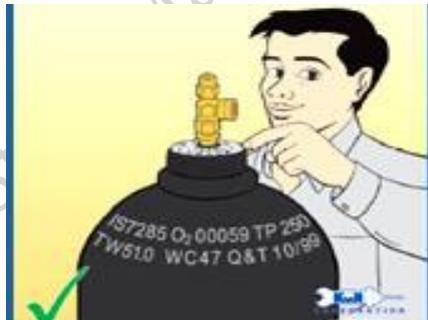
**Fig. 1.9 Checking the expiry date of the cylinder**
