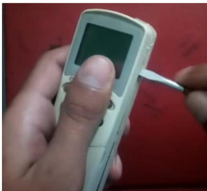
**Fig. 3.41 Removal of battery of remote**
