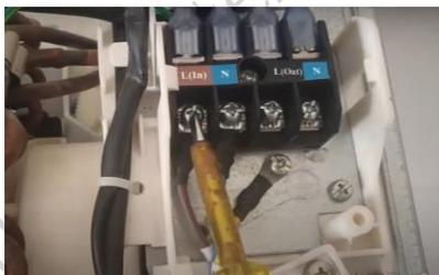
**Fig. 3.22 Connection removal**
