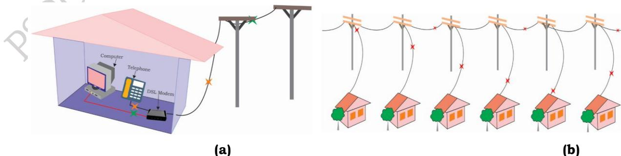
**Fig. 4.4 (a) DSL modem connection distributing the voice and internet signal (b) DSL having a dedicated line for every user**
