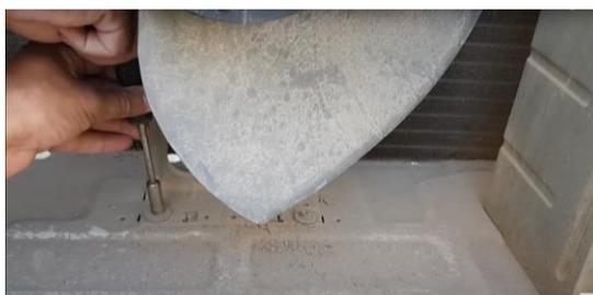
**Fig. 3.5 Unscrewing of fan bolts**
