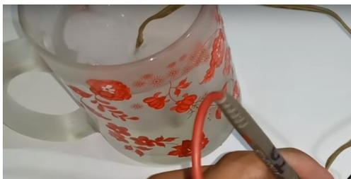
**Fig. 2.85 Temperature sensor in the jug**
