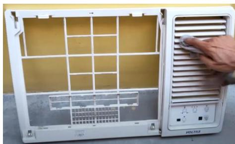
**Fig. 2.60 Clean the front panel of the window AC**
