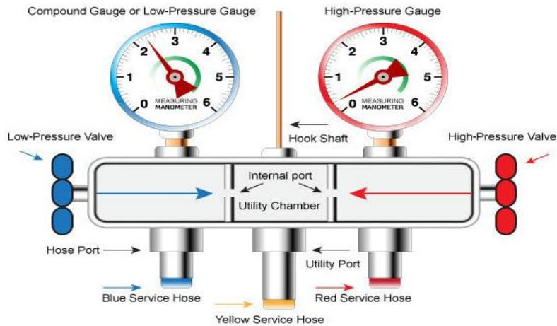
**Fig. 2.6 Manifold gauge**
