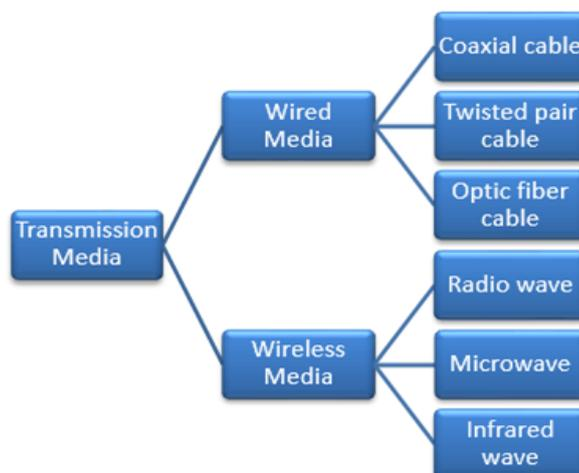
**Fig. 4.10 Classification of Transmission Medium**
