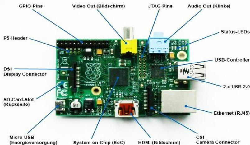
**Fig. 2.2 Parts of Raspberry Pi board**
