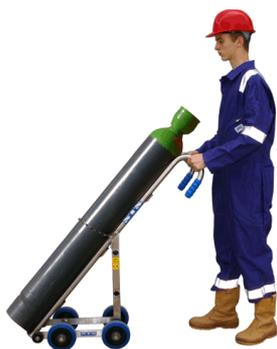
**Fig. 1.16 Right practice to lift the gas cylinder**
