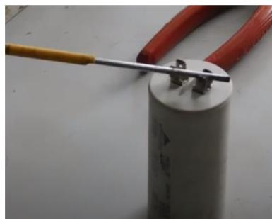
**Fig. 2.93 Capacitor condition check**
