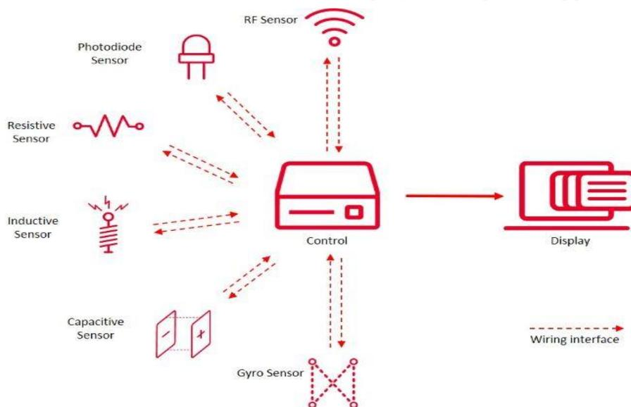
**Fig. 3.12 Sensor wiring to a control system and display**
