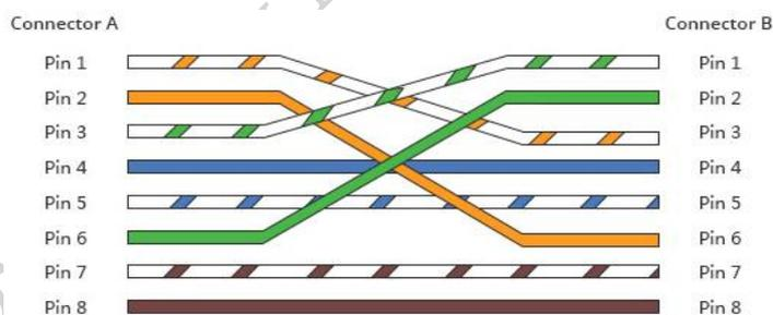
**Fig. 4.18 Crossover cable wiring scheme**
