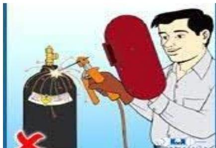
**Fig. 1.3 Wrong way of eradicating leak of refrigerant cylinder**
