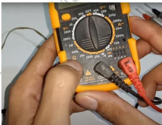
**Fig. 2.83 Multimeter with connected cords**
