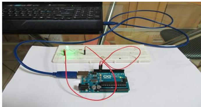
**Fig. 10 Photograph of blinking LED using Arduino**
