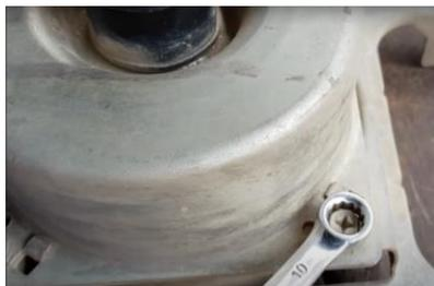
**Fig. 3.10 Removing all bolts of a fan**
