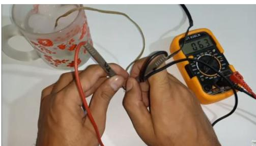
**Fig. 2.86 Resistance of the temperature sensor**
