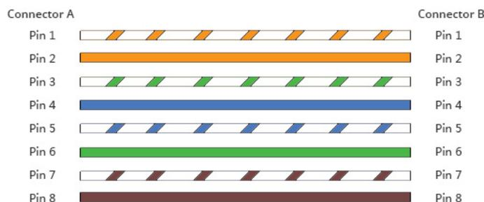
**Fig. 4.17 Straight through cable wiring scheme**
