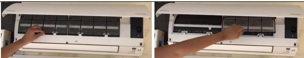
**Fig. 2.33 Unlocking the filter**
