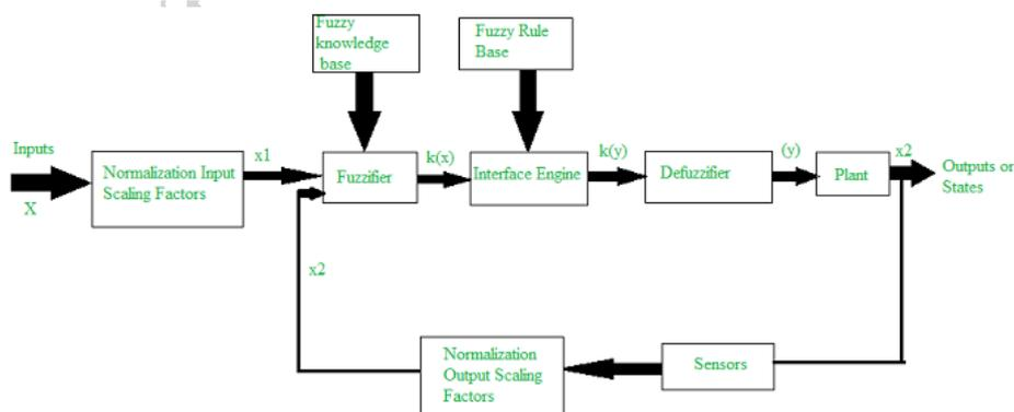
Fig. 1.7 Block Diagram of the FLC for Refrigeration Control
