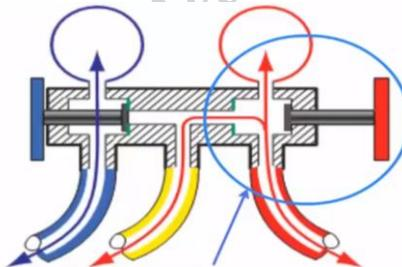
**Fig. 2.12** In this picture, we see that the high side (red) hand-valve is open to either the recovery cylinder or vacuum pump
