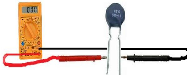
**Fig. 2 Connect the multimeter terminals NTC thermistor leads**
