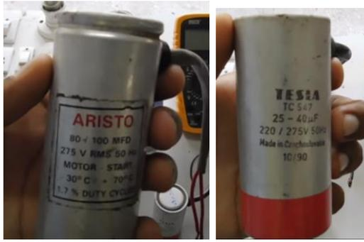
**Fig. 2.91 (a) Specification of start capacitor (b) Specification of running capacitor**
