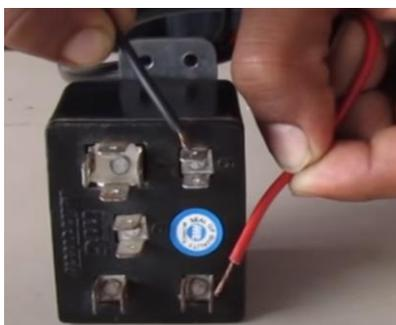
**Fig. 2.89 Touching series lamp to pin 2 and pin 5 of relay**
