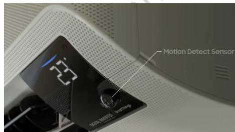
**Fig. 3.14 Motion sensor**
