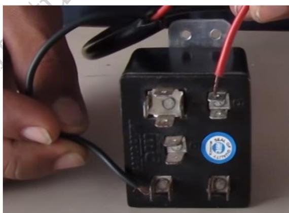
**Fig. 2.90 Touching series lamp to pin 1 and pin 5 of relay**
