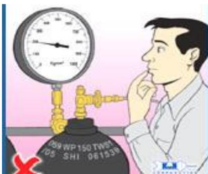
**Fig. 1.8 Avoid overfilling the cylinder**
