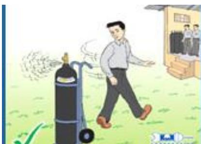
**Fig. 1.10 Placing of leaking gas cylinder to open space**
