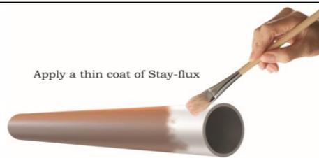
**Fig. 3.38 Flushing using brush**
