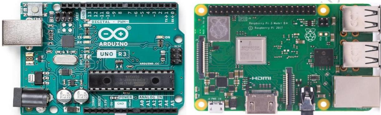
**Fig. 3.2 (a) Arduino UNO Board (b) Raspberry Pi board**
