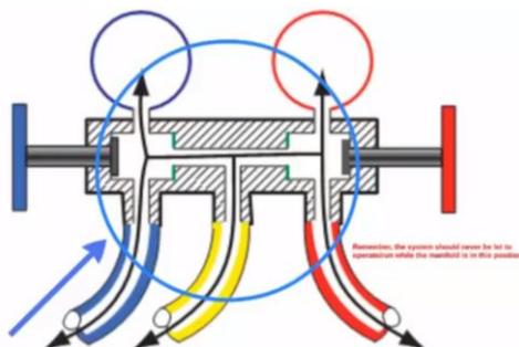
**Fig. 2.13** In this picture, we see both hand-valve is open, usually when in this position it is for either pressure testing recovery cylinder or using vacuum pump
