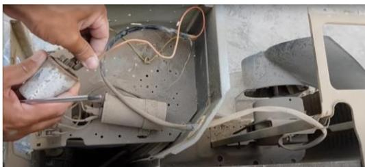
**Fig. 3.7 Removing all the wires of a fan**
