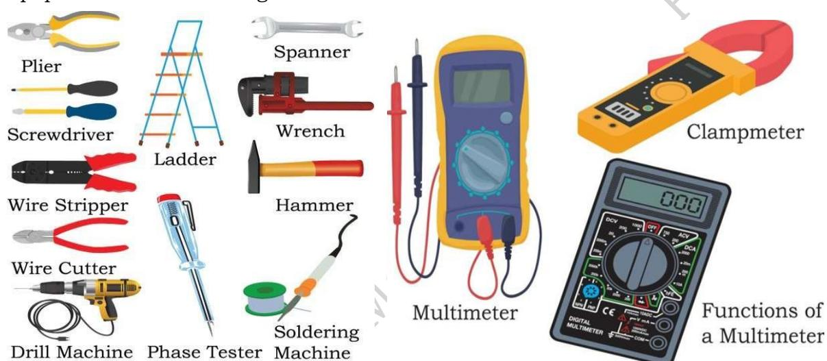
**Fig. 1.1 Common hand tools and equipment**
