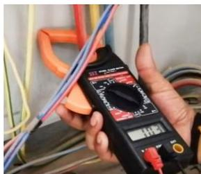
**Fig. 4 Reading on display in clamp meter**
