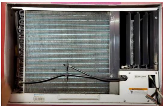
**Fig. 2.57 Clean the temperature sensor**
