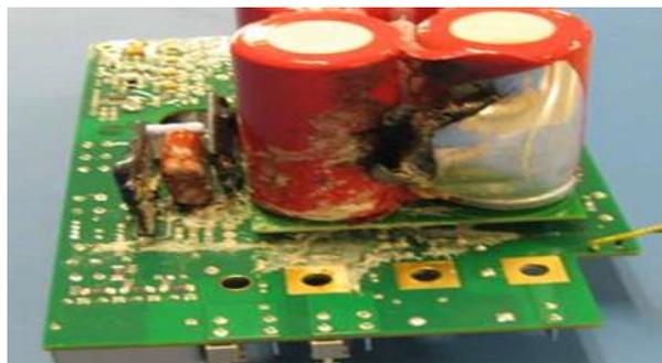
**Fig. 3.11 Old capacitor with the damaged body on the PCB**
