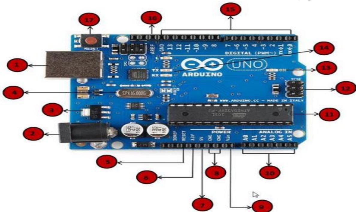
**Fig. 2.3 Arduino Uno board**
