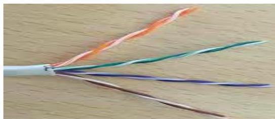
**Fig. 4.13 Unshielded Twisted Pair Cable**
