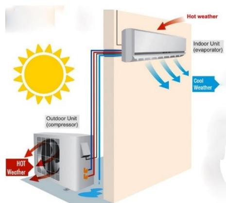
**Fig. 2.1 Setup showing the indoor and outdoor unit of split AC conditioner**
