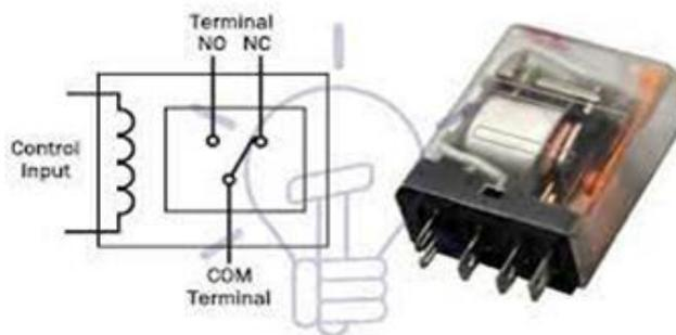
**Fig. 3.17 Voltage Relay terminals**
