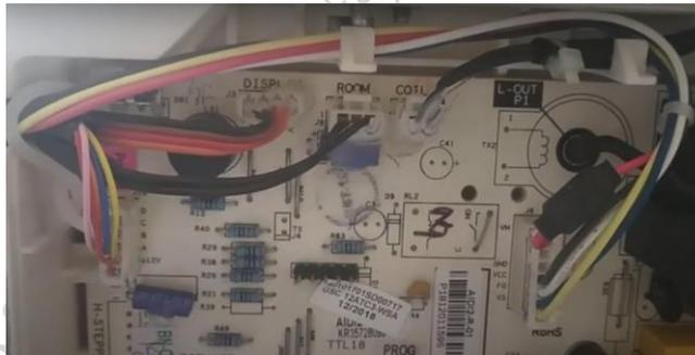
**Fig. 3.33 Detachment of coil sensor terminals**
