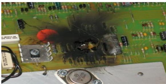
**Fig. 3.7 Power failure in the PCB**
