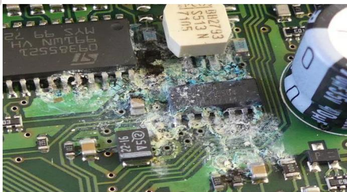
**Fig. 3.10 Environmental Damaged to a PCB**
