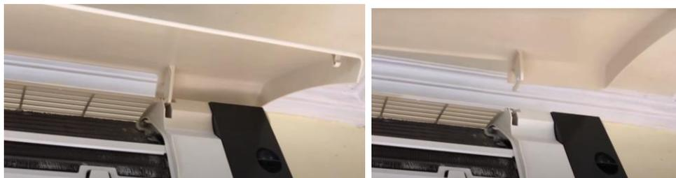
**Fig. 2.21 Sliding the right rotary shaft**
