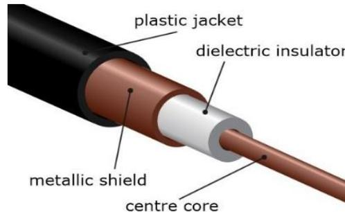
**Fig. 4.11 Coaxial cable**
