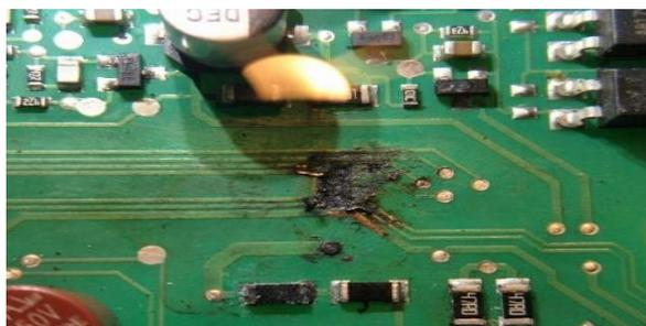
**Fig. 3.5 Trace damage in the PCB**
