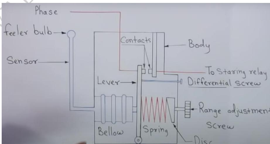
**Fig.2.69 Internal circuit of the thermostat**
