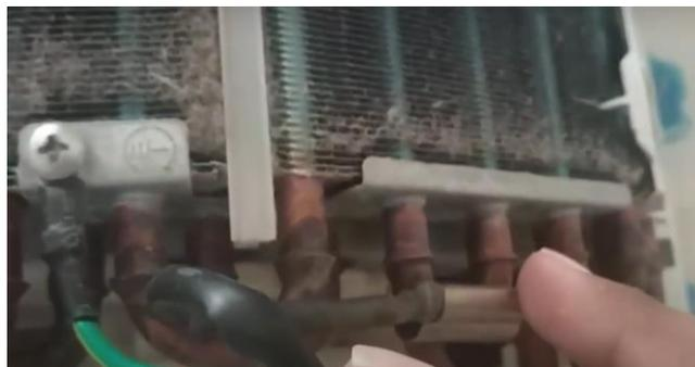
**Fig. 3.34 Removal of coil sensor**
