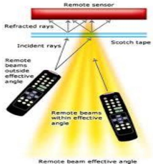
**Fig. 4.23 Infrared light wave used in television remote**
