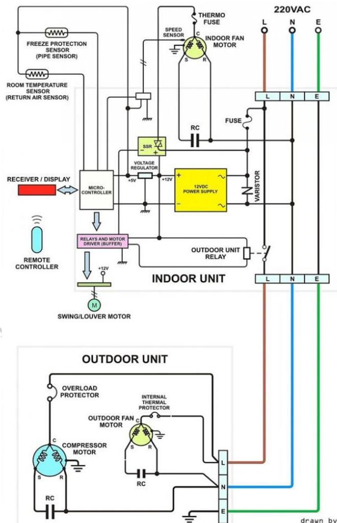
**Fig. 3.2 Circuit diagram of the air conditioner**
