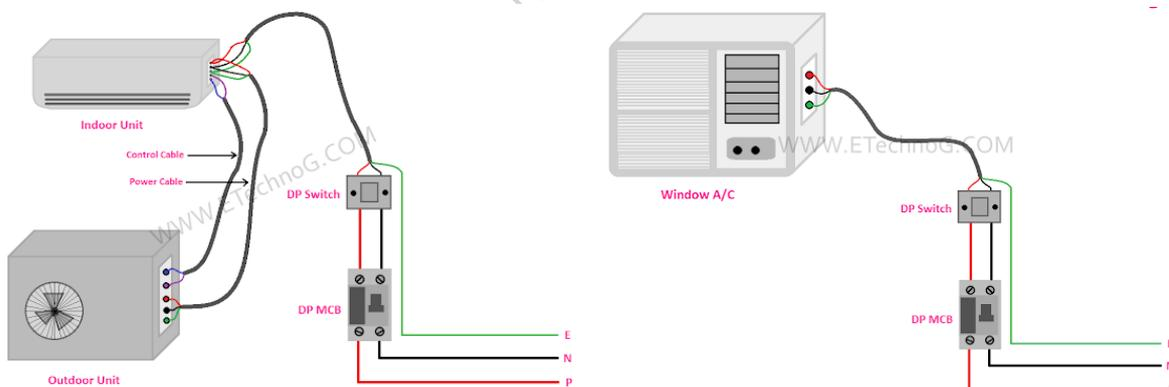
**Fig. 3.1 Block diagram air conditioner (a) Split air conditioner (b) Window air conditioner**
