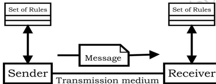
**Fig. 4.9 Transmission of data from sender to receiver through a medium**
