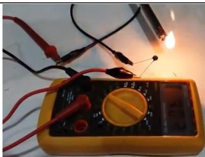
**Fig. 4** Heat around the NTC thermistor
