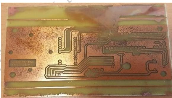
**Fig. 3.6 Poor design of trace in the PCB**
