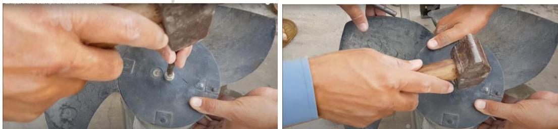
**Fig. 3.9 Loosening of the bolts of fan**
