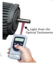
Fig. 1.81 Optical ray coming out from tachometer
