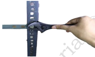
Fig. 1.16 Tighten the nut using an adjustable wrench
