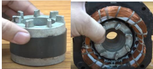
Fig. 3.30 (a) Rotor (b) Rotor placed in the stator
