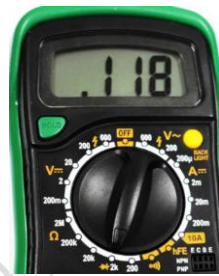
Fig. 1.73 Resistance value in Kilo-ohm
