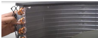
Fig. 1.41 Copper pipe of condenser
