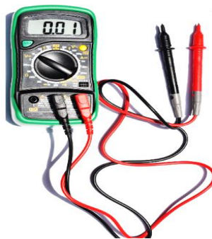
Fig. 1.74 Connecting the red probe to the volt terminal and black probe to the common terminal
