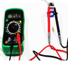
Fig. 1.77 Measuring DC voltage using multimeter
