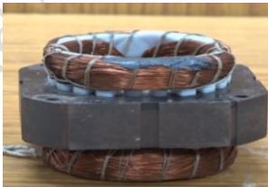
Fig. 3.27 Stator of induction motor
