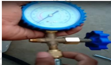
Fig. 2.64 Fix the pipe in the pressure gauge
