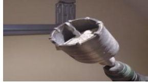
Fig.2.27 Empty the removal coming from the wall
