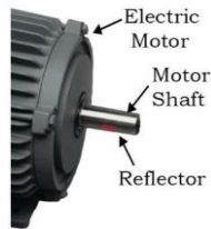
Fig. 1.79 Reflecting tape on the motor shaft
