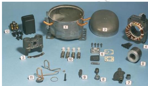
Fig. 3.17: Disassembled hermetic compressor
