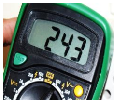
Fig. 1.78 Holding the value in the display using hold button
