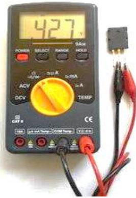
Fig. 1.23 Multimeter probes connected to the MOSFET terminals
