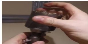
Fig.2.23 Fixing of the drill bit in the power drill
