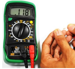
Fig. 1.72 Measuring the resistance of resistor by touching the resistor terminal to the red and black probes
