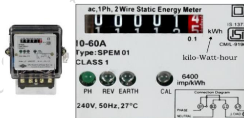
Fig.1.47 Single-phase energy meter
