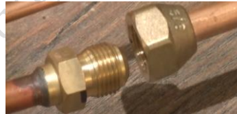
Fig.2.41 Connection of copper pipes
