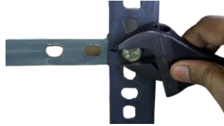
Fig. 1.15 Opening nut using an adjustable wrench
