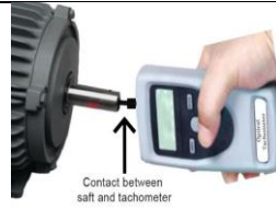
Fig. 1.83 Touch the contact of tachometer to the shaft of electric motor
