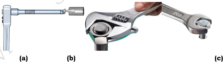
Fig. 1.12 Using (a) socket wrench (b) adjustable wrench (c) open-end wrench
