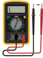
Fig. 1.11 Multimeter in diode mode which shows the reverse bias in diode
