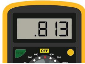
Fig. 1.20 Forward voltage drop in the diode
