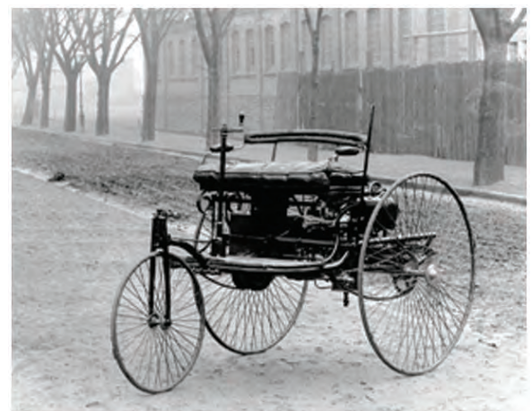
Fig. 1.8: Photograph of the original Benz Patent— Motorwagen, first built in 1885
