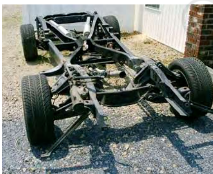
Fig. 3.1: Chassis with suspension and exhaust system
