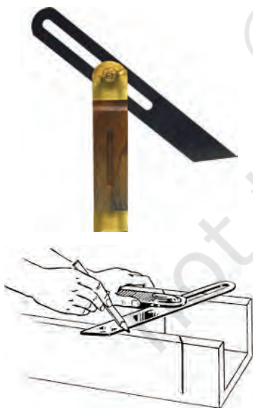
Fig. 4.13: Bevel gauge and its use
