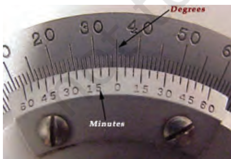
Fig. 4.15: Degrees can be read directly off the main scale, while the minutes are read on the vernier scale.
