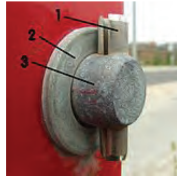
Fig. 2.23: Slotted spring pin (1) and washer (2) used to secure a shaft (3)
