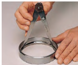
Checking inside groove
