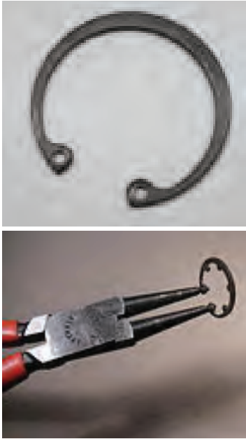
Fig. 2.21: Circlip and circlip plier
