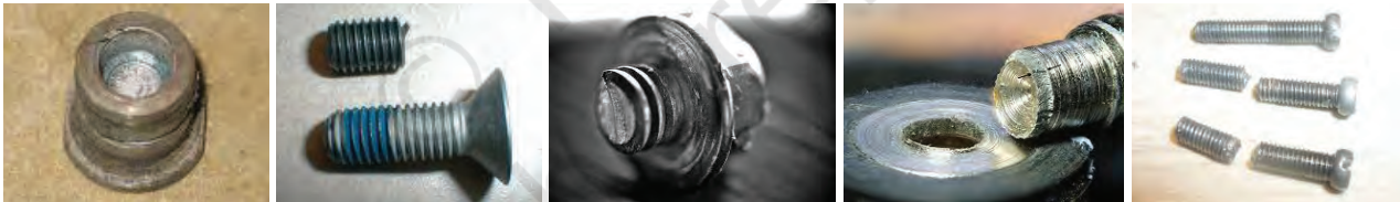
Fig. 2.24: Broken and spoiled screws
