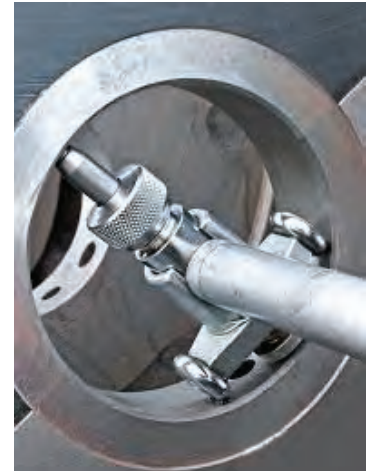
Fig. 4.22: Using bore gauge showing measuring sled
