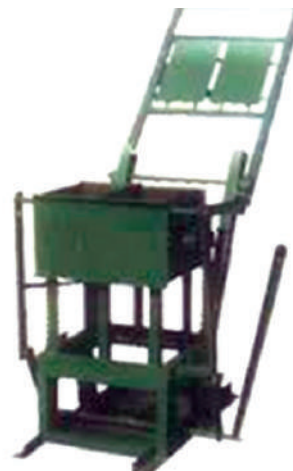
Fig. 4.5: Block casting machine
