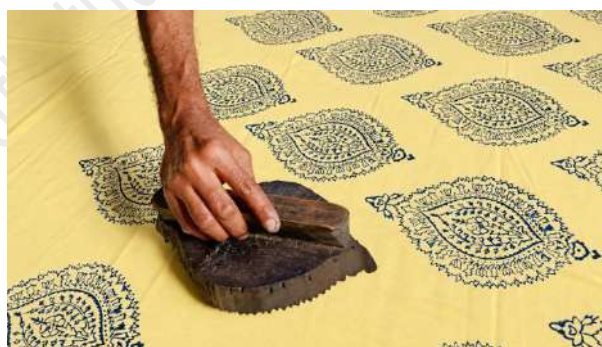
Fig. 4.1: Direct Block Printing
