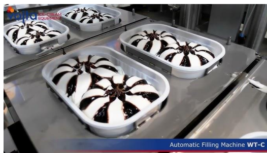
Figure 4.1 Filling of Ice Cream
