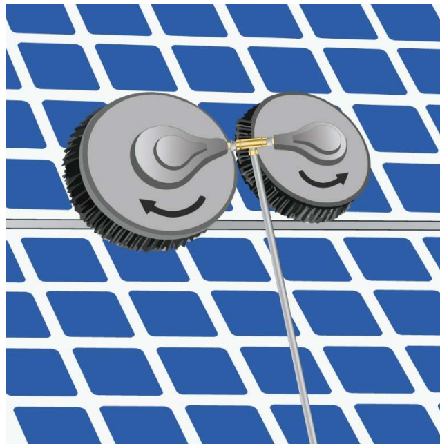
Fig. 10.3: cleaning machines powered by electricity
