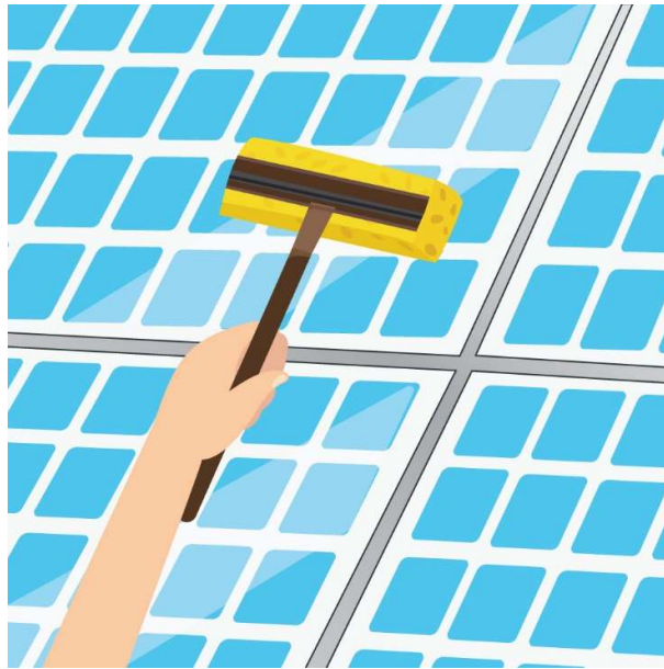
Fig. 10.1: Clean Solar Panel surfaces with a Soft Brush or a Sponge
