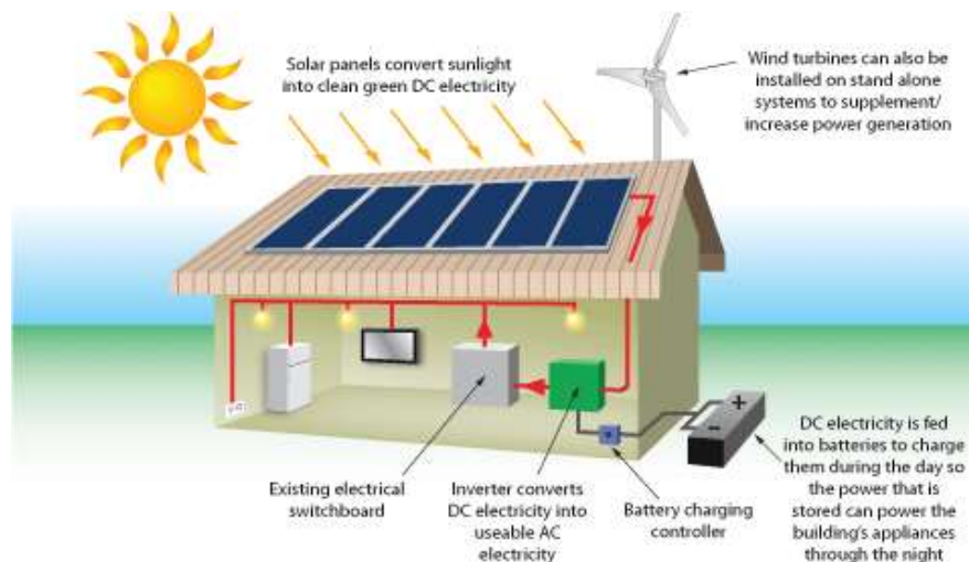
Fig. 6.1: Major system components
