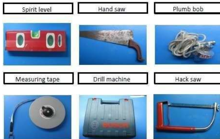
Fig. 6.12: Tools and Tackles for Civil/Mechanical work
