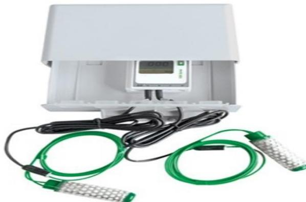
Fig. 5.6: Gypsum block-based sensor
