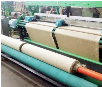
Fig. 2.12: (a) Weaving of Jute on a Power loom (b) Weaving of Jute on a Handloom
