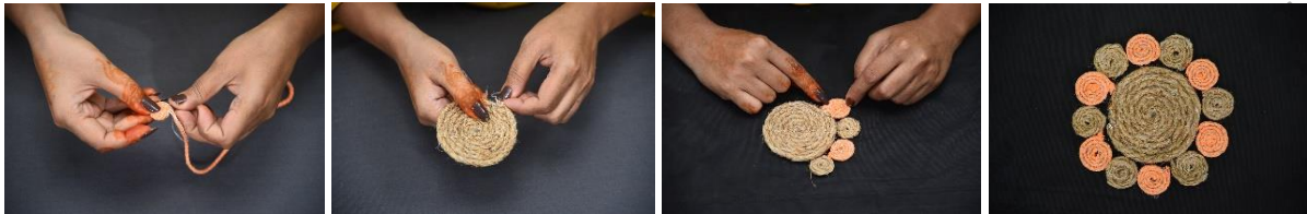
(a) Stitching jute yarn for coiling b) Stitching coils to make costar
