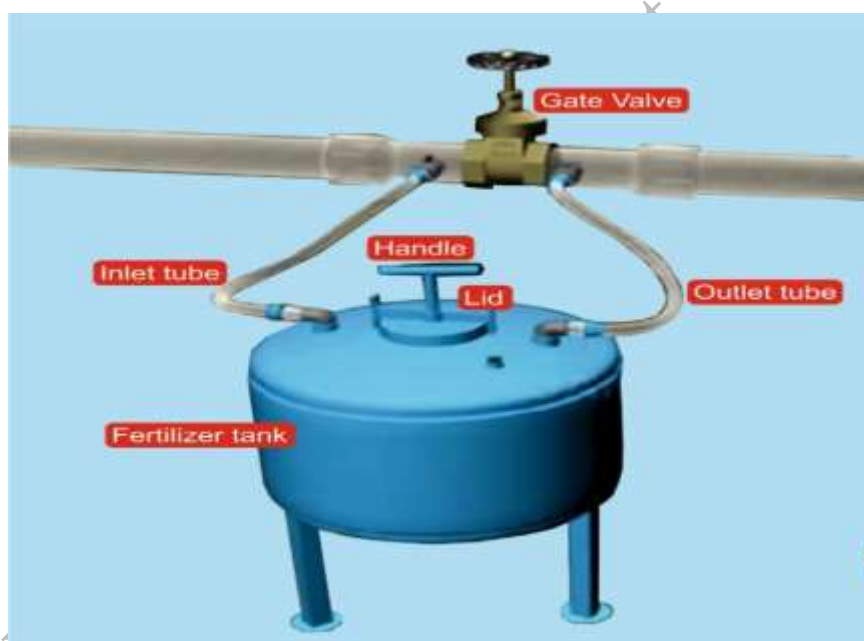
Figure 1.48: Fertiliser tank assembly
