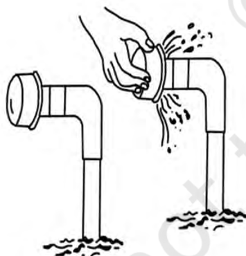
Fig. 3.5: Main or sub-main flushing
