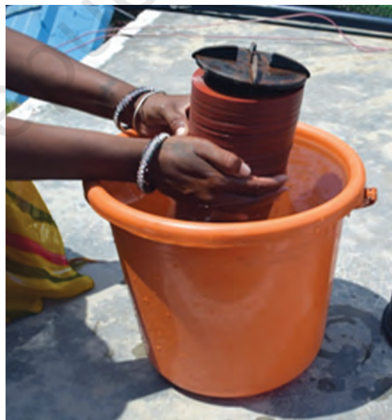
Fig. 3.8: Cleaning of disc filter
