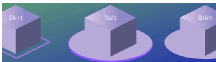
Fig 4.6: Comparison between Skirt, Raft and Brim
