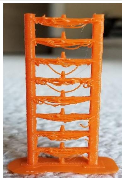
Fig 4.3: Bridging in 3d Printing
