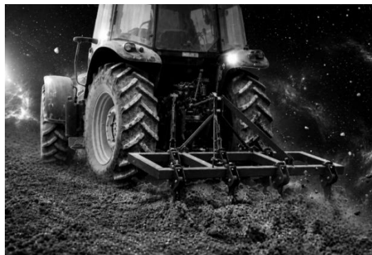
Fig. 2.4: Chisel plough, used to loosen the deeper layer of soil
