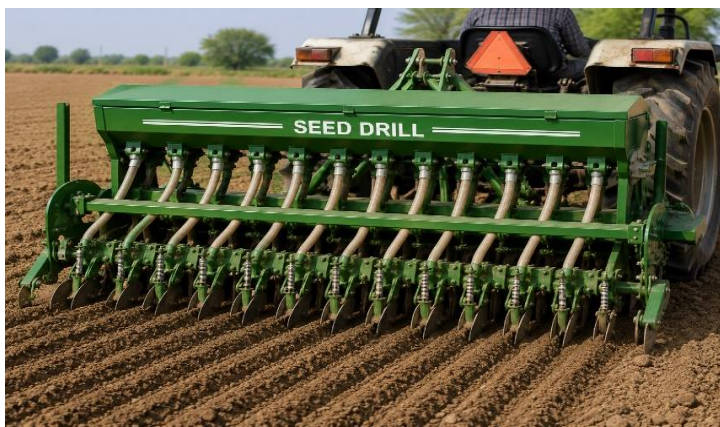
Fig. 2.5: Seed drill, used for sowing seeds uniformly at proper depth and spacing
