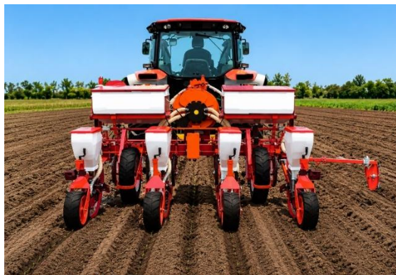
Fig. 2.6: Precision planters ensure accurate seed placement
