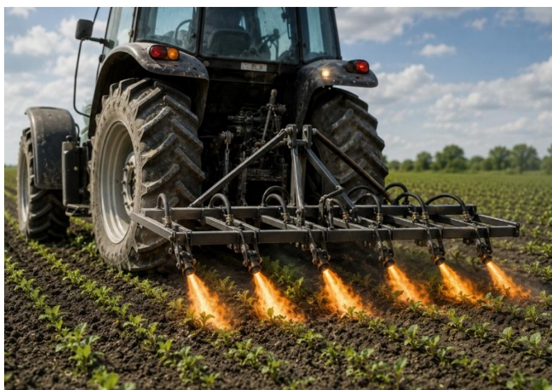
Fig. 2.7: Flame weeder used for chemical-free weed control
