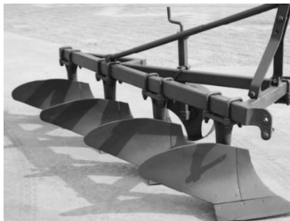
Fig. 2.3: Moldboard plough, used for primary tillage
