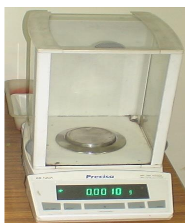
Fig: 2.8: An electronic balance used to measure the mass of an object with high accuracy
