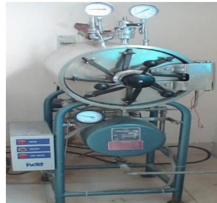
Fig: 2.5: An autoclave used to sterilize nutrient media, glassware, equipment, and other materials
