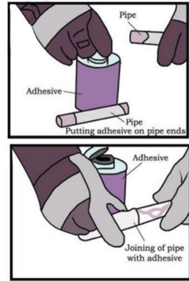
Fig 1.3 Joining of elbow after application of solvent
