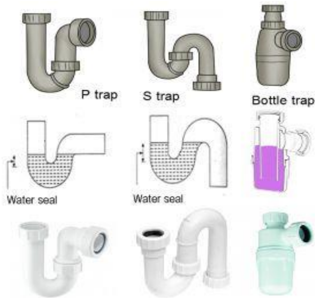
Fig 1.7 Types of Traps
