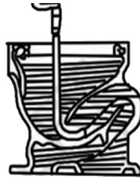
(b) Cleaning the toilet with a snake
