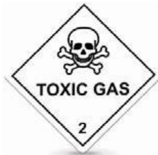
Fig 3.8 Hazardous toxic gas
