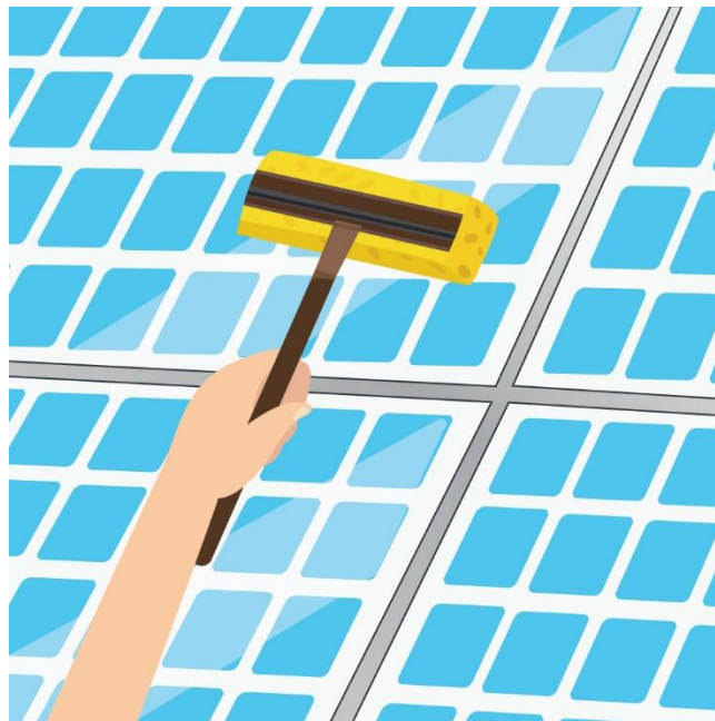
Fig. 2.1: Clean Solar Panels surfaces with a Soft Brush or a Sponge
