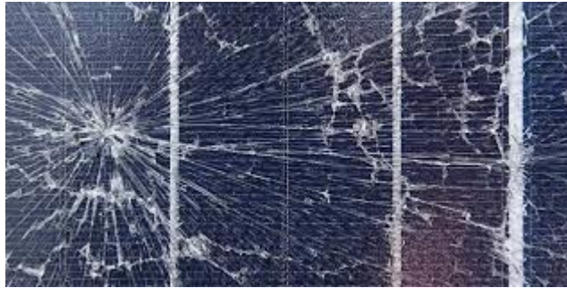
Fig 2.7: Broken glass of solar panel
